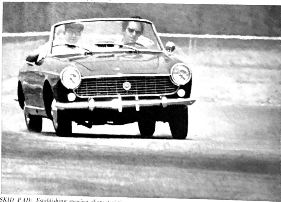
SKID PAD: Establishing steering characteristics.
