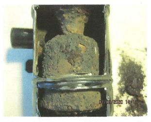
in brass. The factory used brazing on steel to assemble the OEM unit. Soldering brass using low temperature solder is a technique that any handyman, me included, could replicate. Using brass also avoids corrosion inherent in the OEM steel units and their failure characteristics.
